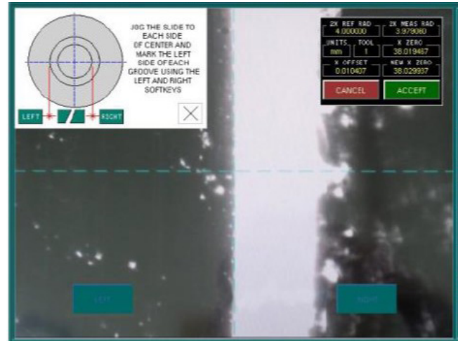
On screen reports, "X Offset" value automatically updated in to tool table
